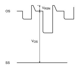
Note 10: Random noise is defined as the standard deviation (sigma) of the output level difference between two adjacent effective pixels under no illumination (i.e. dark conditions) calculated by the following procedure.
