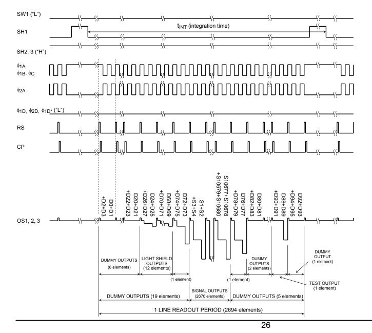
Application Note: Timing Chart (Color 300DPI Mode: Line Clamp Mode) SW2 = "H"
