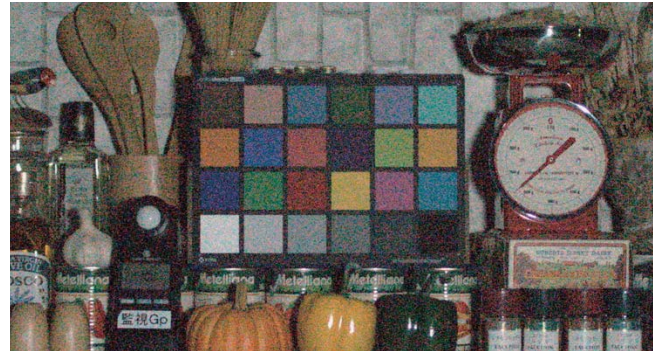
IMX124LQT (the new product) Internal gain 51 dB/ADC 12 bit mode
