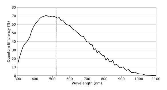
Forge FG-P5G-50S4C Spectral Response Curve
