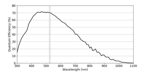
Forge FG-P5G-161S7C Spectral Response Curve
