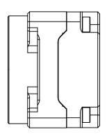
GPIO CONNECTOR-JST BM06B-NSHSS-TBT
