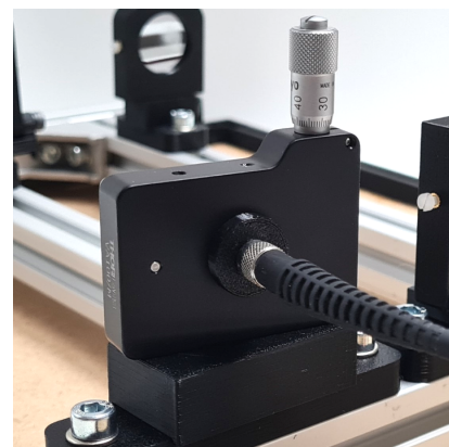
Signal coupling with low-OH optical fiber
