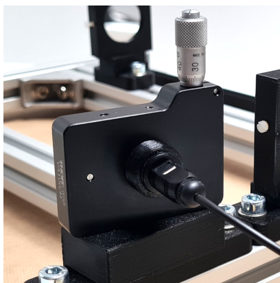
Signal coupling with TOSLINK optical fiber
