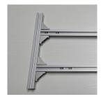
Screw profile D to B and C: Similar to the previous step, two slot nuts are required in the lateral groove of part D and one each in the lateral grooves of parts A and B. Before assembling, however, two slot nuts each must be inserted into the upper groove of parts B and C (modules will be placed here later).
