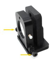
The tilting mechanism consists of a knurled screw SM-3x20-T with a spring SP-5x15 and a plastic washer WA-M3-P. Attach these at the top as shown in the adjacent figure. Screw the knurled screw into the threaded insert until the component holder is approximately perpendicular to the baseplate.
