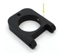
Place the mirror holder 3D-2011 on its baseplate 3D-2090 and fix it with the two cylinderhead screws SM- $3\times25$ . These are simply inserted into the corresponding holes.
