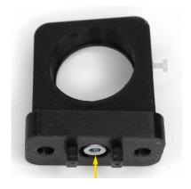
Insert a SM-5x14 cylinderhead screw with a WA-M5 washer from above through the remaining mounting holes. The module is then later screwed to the profile with these.
