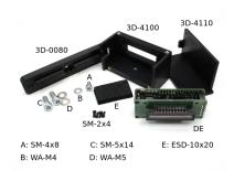
The »3D-\*« components are individually adapted to the component and made from PLA filament using a 3D printer. The step files are available on request and via download.
