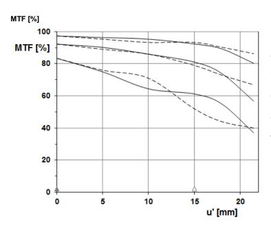
Modulation transfer MTF as a function of the image height (u') and slit orientation. White light. Spatial frequencies R=10, 20 and 40 cycles/mm.
