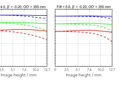
– 10 LP/mm, radial - 20 LP/mm, radial 30 LP/mm, radial --- 10 LP/mm, tangential --- 20 LP/mm, tangential --- 30 LP/mm, tangential
