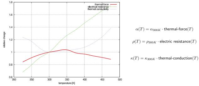
• The device has two ceramic plates, one on the hot and one on the cold side. The values for the thermal conduction shown above do not include the influence of these ceramic plates. The plates have a thickness of  $\leq 1mm$  and a thermal conductivity of  $\geq 15 W/K \cdot m$  which should be used for calculations.
