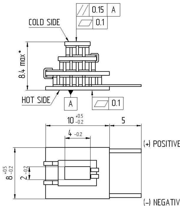
\*Tolerance of the TEC's height for a lot is  $\pm 0.35$  mm
