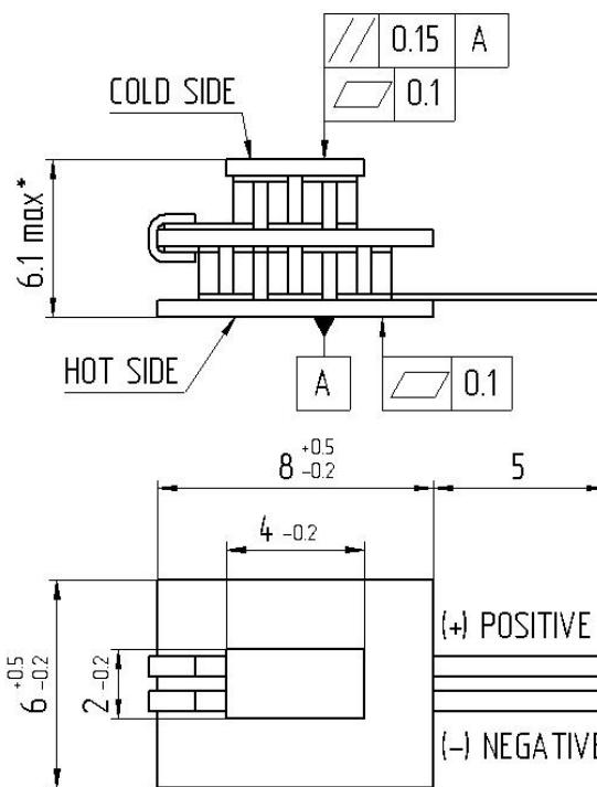
\*Tolerance of the TEC's height for a lot is  $\pm 0.35$  mm
