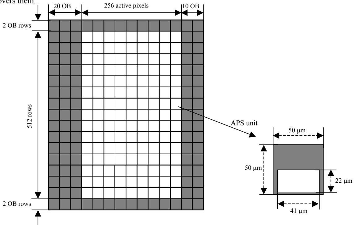
Figure 9. Sensor array and each pixel geometry.
