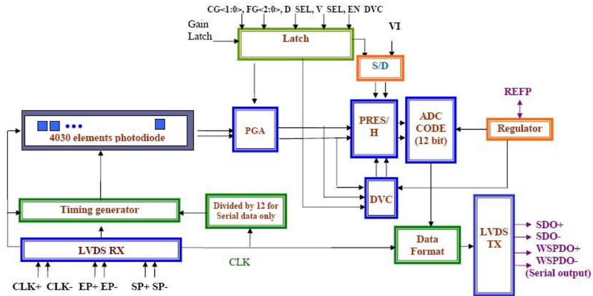
Figure 2. The block diagram of C640 image sensor.
