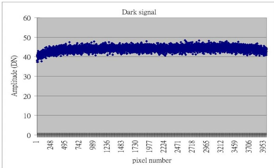
Figure 3. The dark signal of the 4000 pixels
