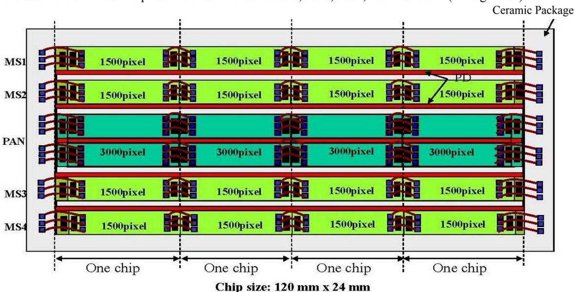
Figure 12. Demonstrate C468 sub-chip diagram in a ceramic package
