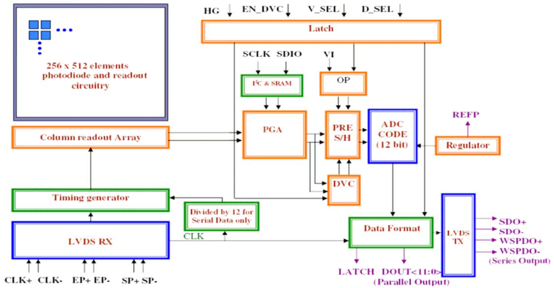
Figure 8. Block diagram of C450 image sensor.
